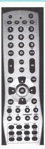
Right Panel. Good contrast for lettering (white on black, black on silver); good inter-key spacing on number buttons and directional buttons, but poor spacing on bottom buttons; character size is too small on some of the smaller buttons.
