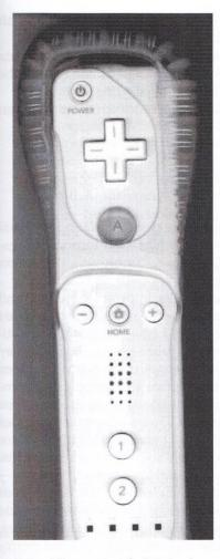
Left Panel. Poor contrast for lettering (gray on white); good use of redundant cues (button size and shape) and inter-key spacing. Plastic covering (see top) around the back and sides of the controller provides an effective grip surface for this controller which requires rapid movement by the user during game play. It also has a wrist strap (not shown).
